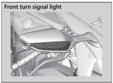
The front turn signal lights uses several LEDs. If there is an LED which is not turned on, see your dealer for servicing.
