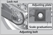
**5.** Turn both adjusting bolts an equal number of turns until the correct drive chain slack is obtained. Turn the adjusting bolts counterclockwise to tighten the
