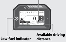
After refuelling more than the reserve amount, the display returns to normal when the ignition switch has been (On) position for about a minute.
