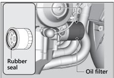
**8.** Apply a thin coat of engine oil to the rubber seal of a new oil filter.
