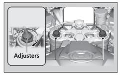
**4.** Turn clockwise to increase spring preload (hard), or turn counterclockwise to decrease spring preload (soft).
