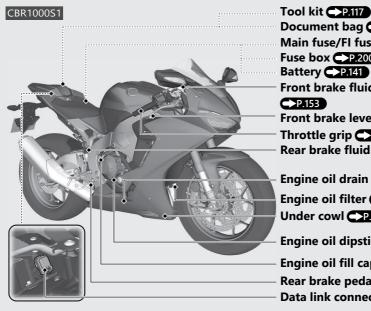
Document bag P.117 Main fuse/FI fuse →P.201 Fuse box P.200 Battery P.141 Front brake fluid reservoir **◯** P.153 Front brake lever P.166 Throttle grip P.164 Rear brake fluid reservoir P.153
