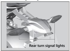
The rear turn signal lights uses several LEDs. If there is an LED which is not turned on, see your dealer for servicing.
