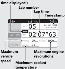
The lap time data include lap time, maximum vehicle speed, maximum engine revolutions, maximum coolant temperature, maximum acceleration, maximum deceleration, maximum left bank angle and maximum right bank angle.
