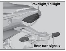
The brakelight, taillight and rear turn signals use several LEDs.
