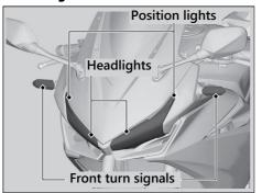
The headlights, position lights and front turn signals use several LEDs.
