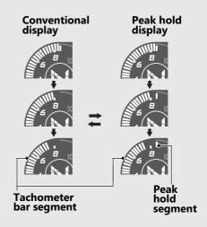
The peak hold segment keeps to show the maximum engine RPM temporarily.
