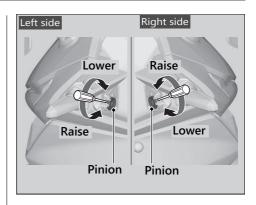
Other Adjustments Adjusting the Brake Lever
