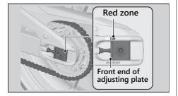
Drive Chain ► Checking the Drive Chain Slider
