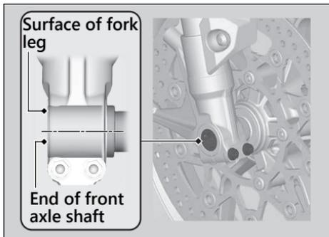
4. Tighten the right axle pinch bolts to hold the axle.
