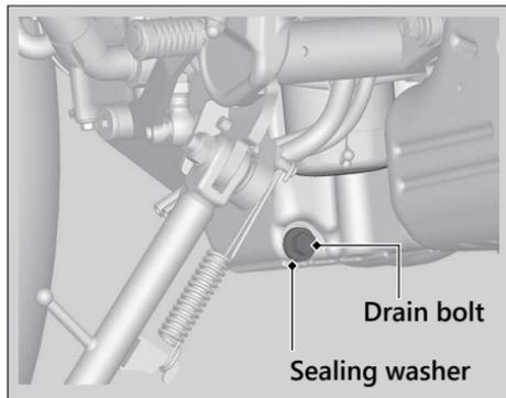
5. Remove the oil fill cap/dipstick, drain bolt, and sealing washer to drain the oil.
