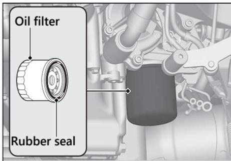
7. Apply a thin coat of engine oil to the rubber seal of a new oil filter.
