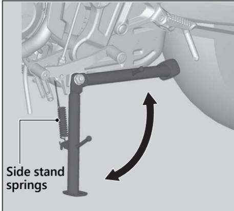
1. Check that the side stand operates smoothly. If the side stand is stiff or squeaky, clean the pivot area and lubricate the pivot bolt with clean grease.
