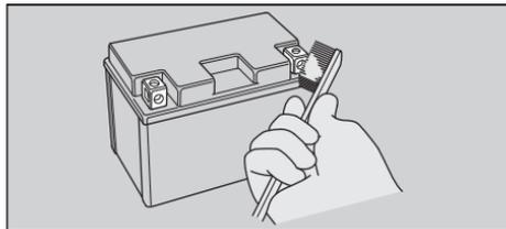
4. After cleaning, reinstall the battery. The battery has a limited life span. Consult your dealer about when you should replace the battery. Always replace the battery with another maintenance-free battery of the same type.
