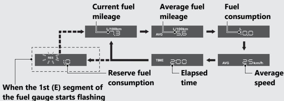
When the 1st (E) segment of the fuel gauge starts flashing, the current fuel mileage, average fuel mileage, fuel consumption, average speed and elapsed time to the reserve fuel consumption.
