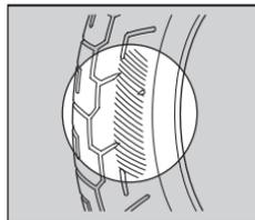
Inspect the tyres for signs of abnormal wear on the contact surface.
