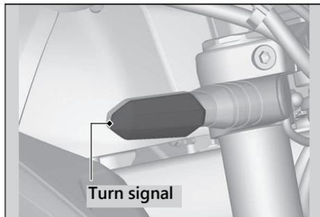
The front and rear turn signals uses an LED. If there is an LED which is not turned on, see your dealer for this service.
