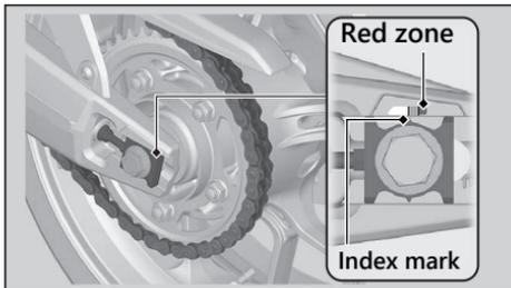
**Checking the Drive Chain Slider**
