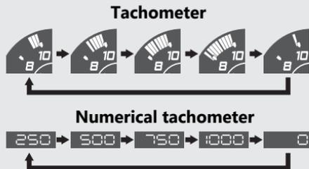
Example: REV indicator blinking fastest
