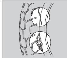
Inspect the tyres for cuts, slits, or cracks that exposes fabric or cords, or nails or other foreign objects embedded in the side of the tyre or the tread.
