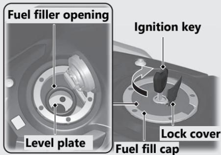
Do not fill with fuel above the level plate.
